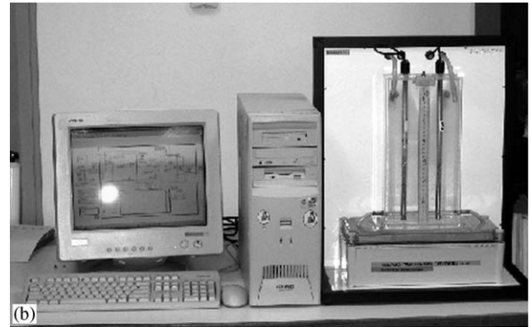
Fig. 6. The coupled-tank liquid-level control system: (a) Schematic diagram; (b) experimental setup.
