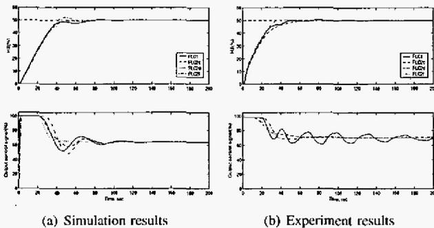
Fig. 10. Step responses when there was a 1 sec transport delay
