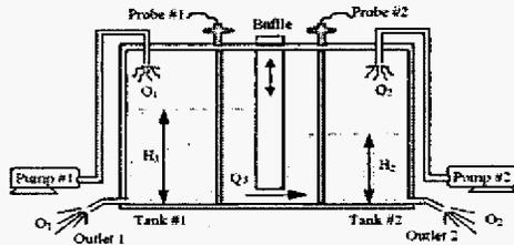
Fig. 5. The coupled-tank liquid-level control system
