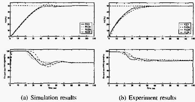
Fig. 7. Step responses when the setpoint was 15 cm
